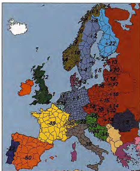
Transformation parameters from national heights to UELN heights in Europe (in cm)
