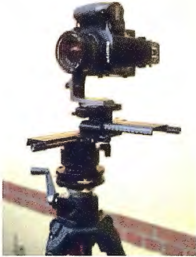
Fig. 1: Digital camera Kodak DCS 645M mounted on panorama
