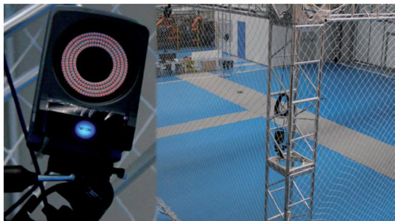
Figure 5. VICON tracking system and indoor testbed in CATEC
