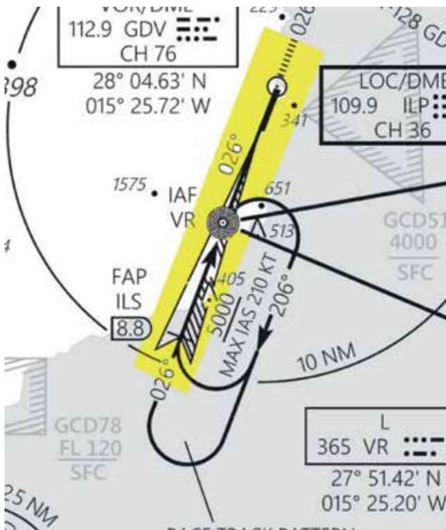
Figura 8. Instrumental Landing System (ILS)
