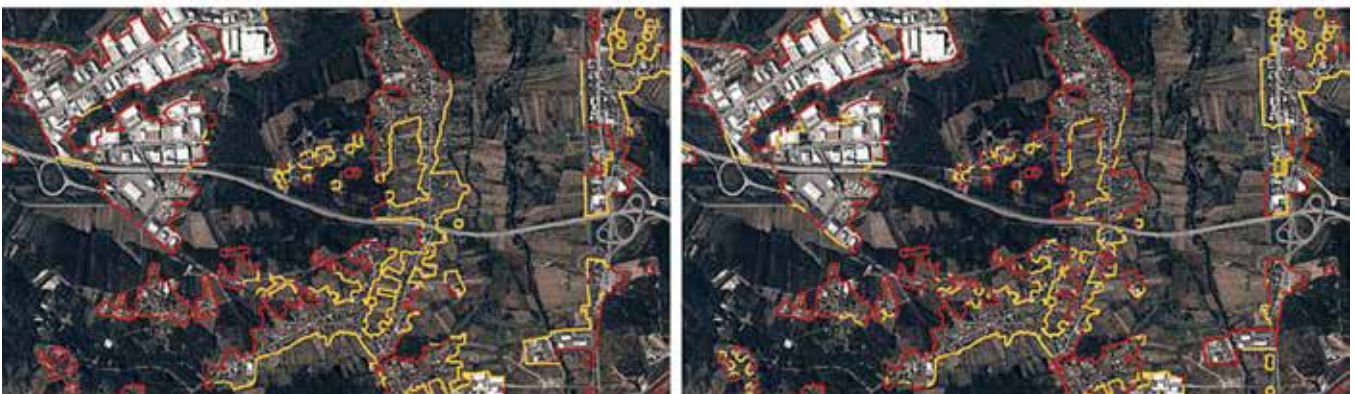
Figure 7. CAE (top) delimits the built-up areas and classifies them in three classes according to the present and type of buildings enclosed, while CIAE (bottom) classifies the interface between the built-up areas of CAE and the surroundings according to the proximity of vegetation; the differences between the structural CIAE (left) and conjunctural CIAE (right) are due to different methodologies and input data (COS and COSc respectively). Orthophotos in true colour shown is the background to provide context
